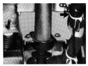
Failure to properly route and secure a wiring harness after repair can result in unwanted squeaks, rattles or damage to the harness and other parts of the vehicle electrical system. Damage to the harness, if undetected, may result in short circuits and under some cirumstances may result in an electrical fire.
